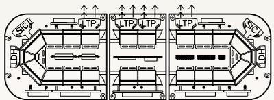
**#5421LED** 20 M-Tech® LED heads, two strobe intersection clearing lights, four front lower takedown/pursuit lights, two alley lights, two front & two rear lower LED heads, lower LED directional arrow assembly
