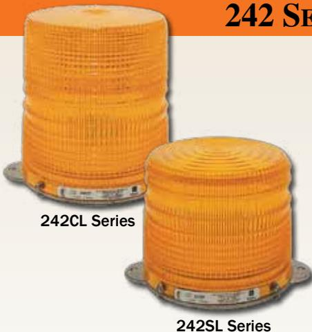
The 242 Series offers a patented LED diagnostic indicator, a photocell for automatic "night" mode switching and field selectable flash patterns of quad flash, double flash, or single flash via an internal jumper. The modular circuit is completely encapsulated for increased shock and weather resistance. The rugged die-cast aluminum base is protected with a powder coat finish. RFI protection is standard. Ships complete with mounting hardware and instructions.
