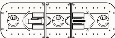
**#8402HSL** One halogen rotator, two fast halogen rotators, two large V-mirrors, two small V-mirrors, four 4.5" linear strobe heads, one 4-head strobe pack
